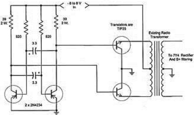
Fig. 3. Multivibrator Plus NPN Power Stage
