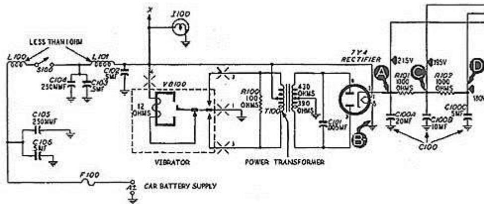
Fig. 1. Philco Model 802 Power Supply
