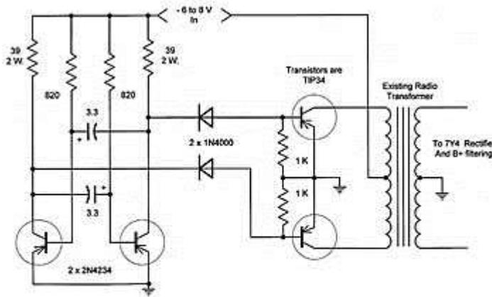
Fig. 4. Final Circuit for Vibrator Substitute
