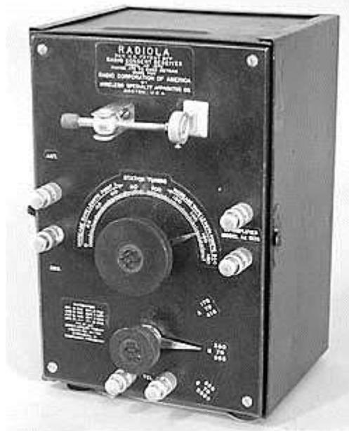
Fig. 4. The exterior of the restored AR-1375 is virtually indistinguishable from the original — except for small blemishes associated with the filling of two holes (see text).
