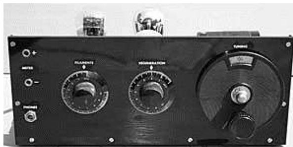
Front panel of my homebrew Colpitts receiver has meter jacks (J3 & J4) at top left, phones/speaker jack (J5) below them. Controls left to right are; filament on/off-rheostat (R7), regeneration (R3), and tuning (C2A).
