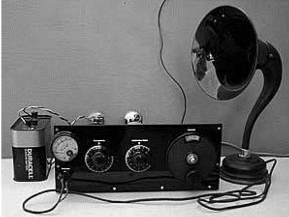
With antenna and B+ supply connected, a 6-Volt lantern battery for filament power, and horn speaker and filament voltmeter plugged in, the set is ready for operation.
