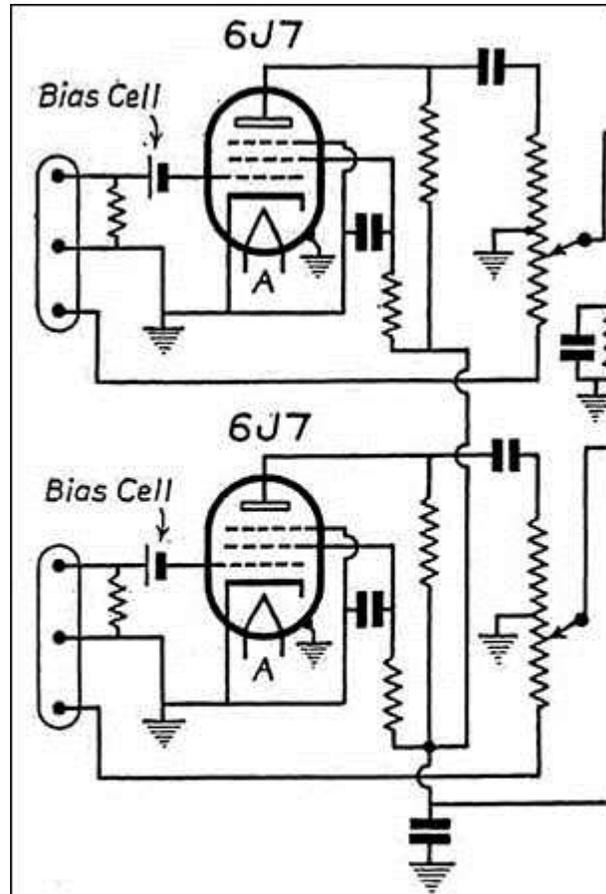
Bias cells as used for grid bias in input circuits of 1936 Lafayette amplifier design.
