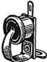
Designed to furnish initial bias for RF, IF and AVC tubes. Size, only  $1\frac{1}{32}$ " x  $\frac{5}{8}$ ". Noiseless; non-reactive at audio frequencies. Provides a no-current potential of 1 Volt  $\pm$  10%. Cells may be used in series for higher bias voltage. These cells greatly eliminate distortion caused by conventional bias arrangements.
