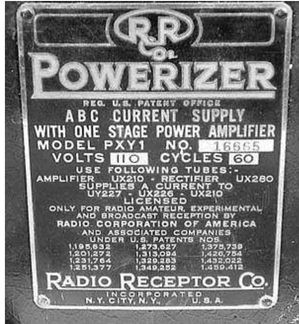
Fig. 2. Second ID plate confirms that this unit is intended to power external 226 and 227 tubes.
