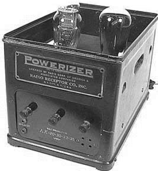
Fig. 1. The Radio Receptor Co. Powerizer. Output panel has speaker jacks, binding posts for "B" voltages, and a 4-pin socket for filament voltages
