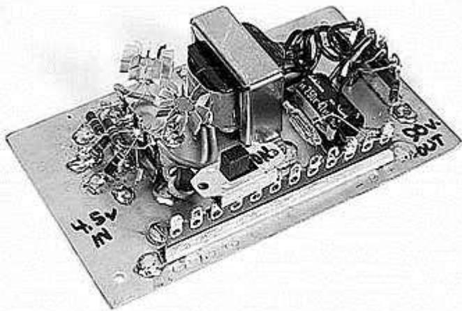
The power inverter circuit.
