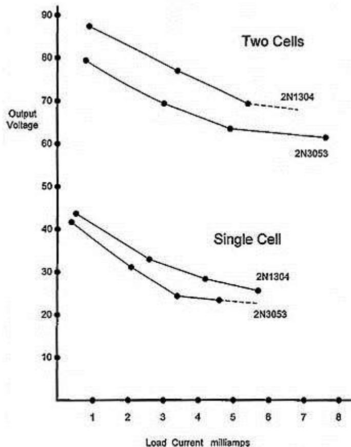
Fig. 1. Power drain curves from the original D-Cell article.
