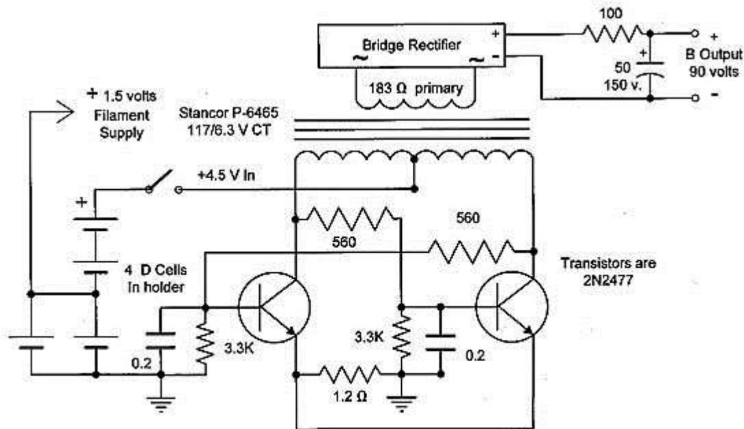
Fig. 2. Power inverter circuit operates on 4.5 volts. 1.5-volts, from two paralleled cells, is tapped off for receiver filament circuit.
