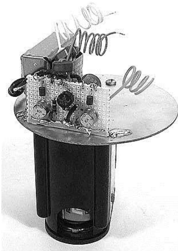
Fig. 4. Two-Cell Power Supply for a Two-Tube Receiver
