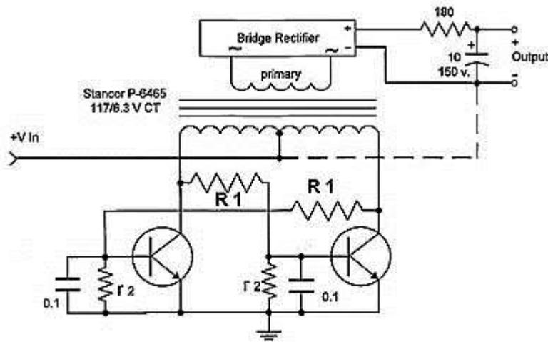
Fig. 2. The Simple Power Inverter (See Text)
