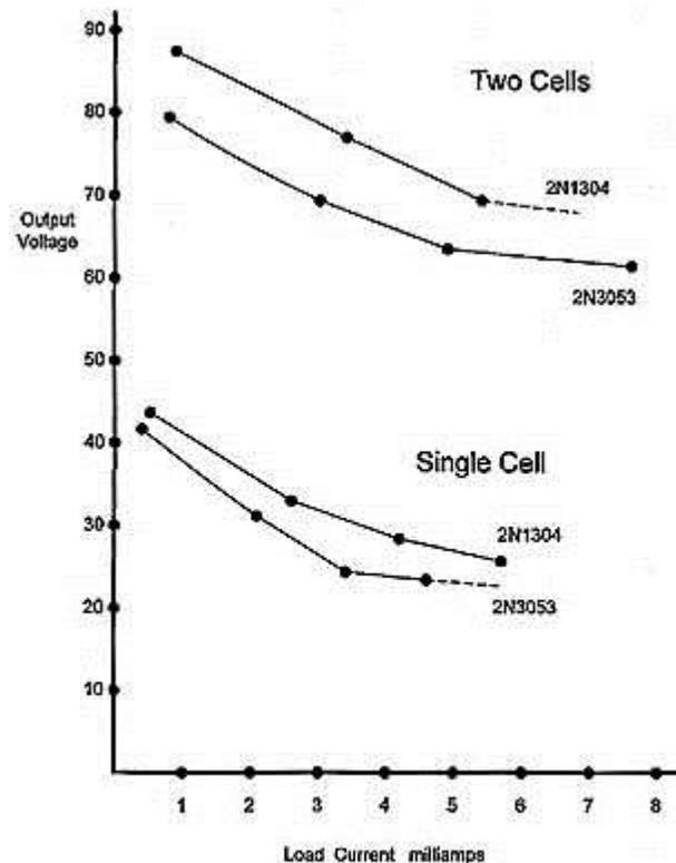
Fig. 3. Test Results With Both Silicon and Germanium Transistors
