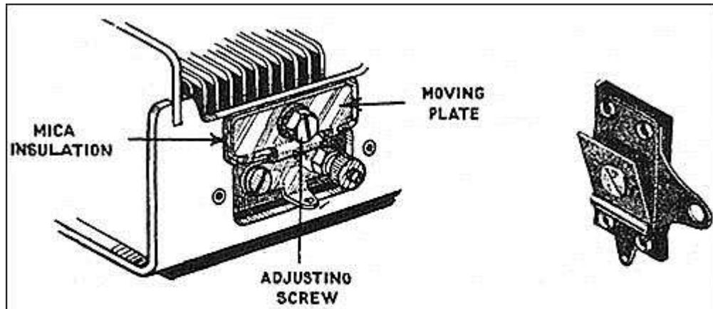
Figure 1. Trimmer capacitors as mounted on variable capacitor frame (left) and mounted individually.
