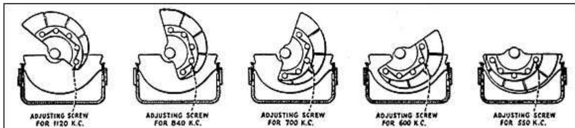
Figure 2. Slotted end plate as might be found on each section of a ganged capacitor. Set screws are provided for adjustment at five different positions.
