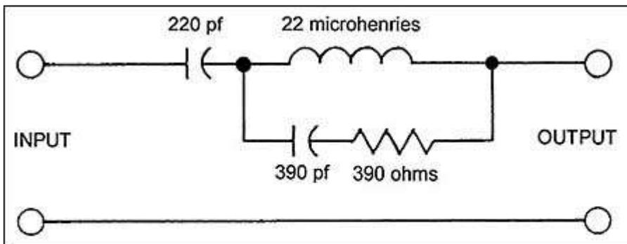
Figure 4. Circuit of a typical dummy antenna.
