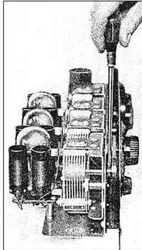
Figure 3. Loosening set screw to adjust position of an individual variable condenser in a group that is ganged by metal bands.
