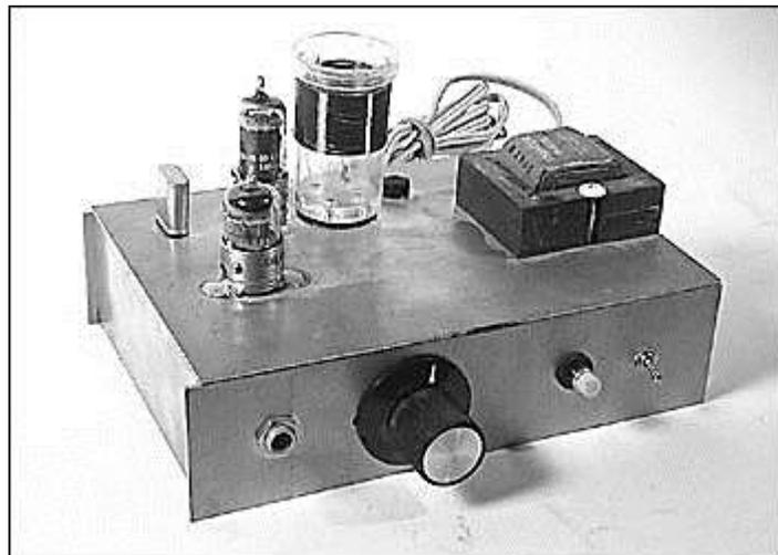
The completed broadcast band transmitter. See text for tank circuit values.
