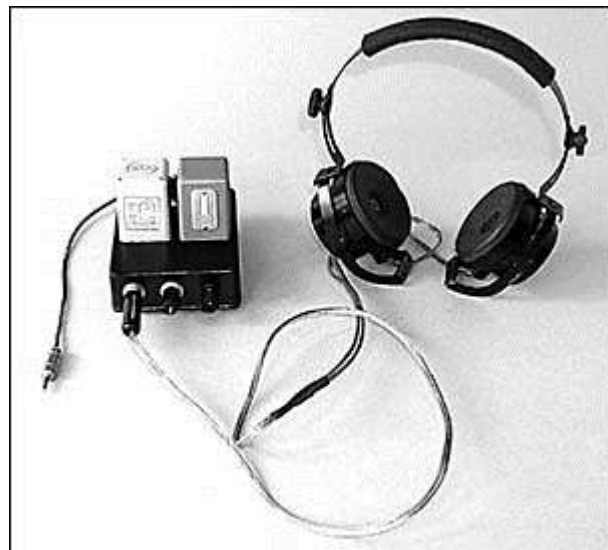
Fig. 4. RCA balanced-armature phones, with matching transformer.
