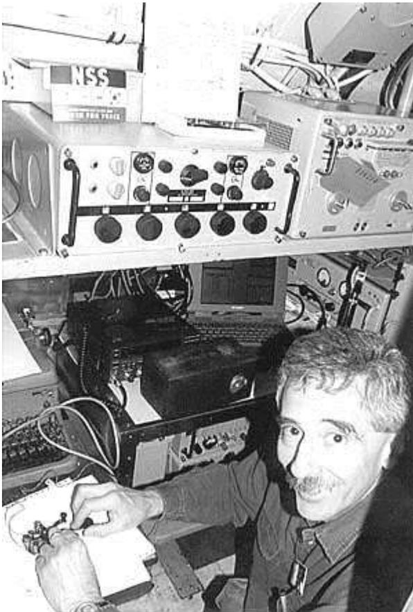
Payoff time! With the RT-618 and AM-3007 reinstalled in Albacore's radio room, Alex establishes a 20-minute CW contact with UA1CJX in St. Petersburg, Russia.
