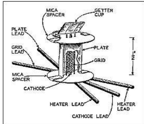
Internal construction of the 955 triode.
