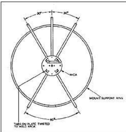
The Dumet rods that would become contact pins were temporarily welded to metal support ring during construction of tube (see text).
