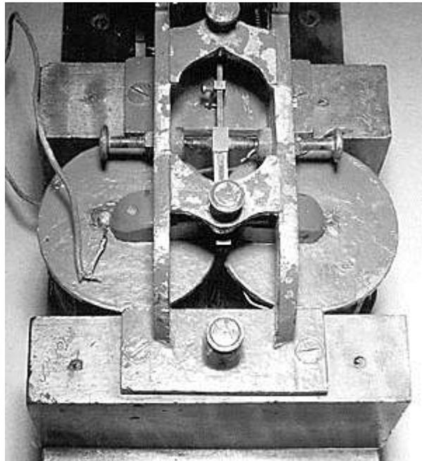
View looking straight down at coil tops shows pen lever in its pivots
