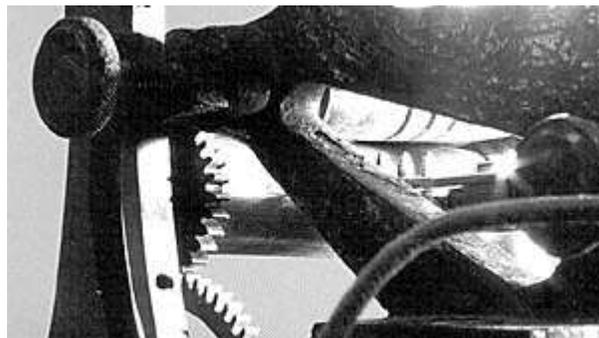
Triple-grooved roller, and the three steel pens directly beneath it, are visible through slot in register frame.
