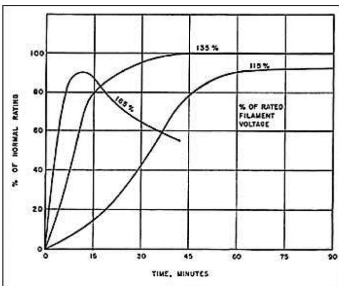
Summary of data accumulated by author on rejuvenation of thoriated tungsten filaments. Best results are obtained at 135% of rated filament voltage. At 115%, rejuvenation time is very significantly increased; at 105%, the tube is quickly destroyed.
